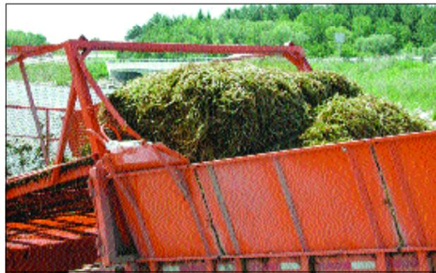
The weed harvester used on Sauk Lake is capable of cutting a path that is six feet deep and nine feet wide. Under ideal conditions, the harvester can cut and transfer 1000 pounds of weeds onto its transporter within 15 minutes. The transporter when full then transfers the harvested weeds onto a trailer. The weeds are then brought to local farmers who utilize them for agricultural fertilizer.
